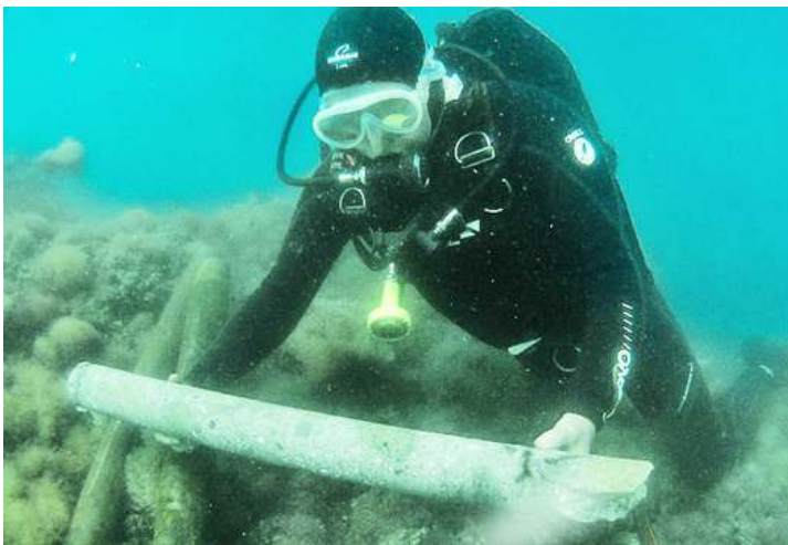
Above: A researcher collecting a Roman concrete sample near Naples, Italy.
